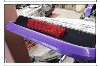
4. If installing the stock bumper, or aftermarket bumper, rivet it into the desired location. This kit will not use the stock snow flap. Once the bumper is installed, finish riveting the Tunnel Cap onto the sides of the tunnel and make sure Tunnel Cap is riveted to both the tunnel and the rear bumper.
