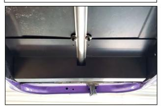
3. Slide the bottom half of the Tunnel Cap Kit into the tunnel first, then slide the top half over the bottom cap. Lay the tail light harness guide over the harness. It will need to be trimmed to fit inside the bottom tunnel cap. Once cut, install onto the bottom of the tunnel.
