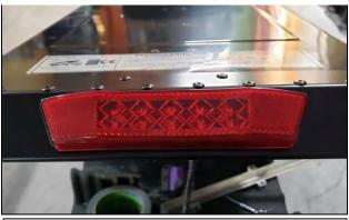
2. Install the taillight onto the top Tunnel Cap using the stock mounting bolts. Be sure to route the tail light harness through the top cap and plug harness into the tail light.
