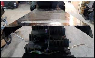
1. Remove the seat, tail light harness guide, tail light, tail light mounting bracket, and snow flap (Remove rear bumper if shortening tunnel) Mark location that you want to cut. Measure twice and cut once. Using a circular saw, execute a smooth continuous cut across the tunnel. Use an air saw cut the remaining tunnel side material to allow the tunnel to separate.
