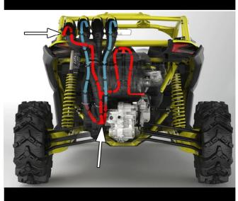
2. Install the Blow Hole by slipping the silicone over the clutch cover exhaust duct first and then slide the top silicone over the upper snorkel duct.
