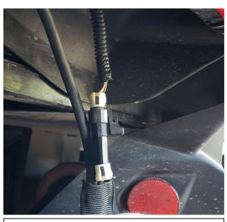
4. Locate the factory tail light connector and plug Blow Hole directly into the tail light as shown. This model of Blow Hole WILL BLOW HOT AIR OUT of the clutch cover.
