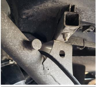
3. Route the wiring harness over the cage as shown and proceed to route wire up towards the tail lights. Be sure to route wire so it does not rub or chafe. Use wire ties if needed.
