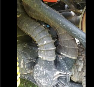
1. Remove clutch exhaust duct tube between the clutch cover and snorkel by loosening the clamps on both ends of the duct hose. This clutch duct tube will not be used. Keep the stock hose clamps for later use.
