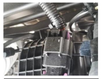
3. Unplug tail light harness connector and plug in Blow Hole connector in line. Properly route and secure wires and connectors with cable ties as needed to prevent damage.
