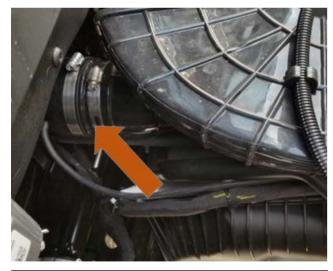
1. Locate the clutch housing intake duct hose. Loosen the clamp holding the hose connection together and separate the intake duct hose from the plastic connector. Leave plastic connector in place with hose connection.
