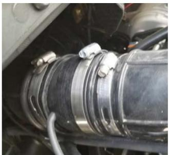
2. Install the Blow Hole onto the clutch housing intake duct hose plastic connector as shown. Then install the intake duct hose onto the Blow Hole assembly. Tighten both clamps.
