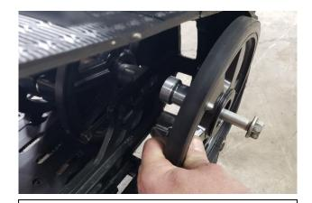
6. Bolt outer wheel into axle as shown. Be sure the standoff is toward the inside of the wheel and the bolt is directly against the wheel. Apply Loctite and leave bolts loose till track is aligned.
