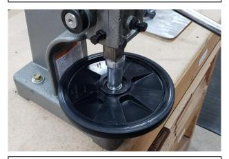
3. Use a press to install standoff assembly onto the stock rear wheel as shown. Be sure standoff is on the snap ring side. Press bearing to shoulder.
