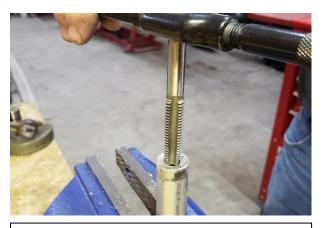
2. Using a M12x1.75 Tap, carefully tap the stock rear axle as shown. Make sure to do this carefully. Once finished, remove all burs and shavings from shaft.
