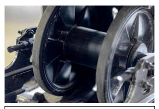
1. Remove the stock rear wheels by loosening the track adjustments bolts and remove the rear axle bolt. Remove the plastic center collar and discard. Remove track adjustment blocks and drill the adjustment collar hole out to 3%"
