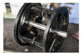
5. Bolt second Tough Wheel onto stock axle as shown. Tighten connector bolts. Install Tough Wheels into rear skid in stock location. Align track adjustment collars with skid windows.
