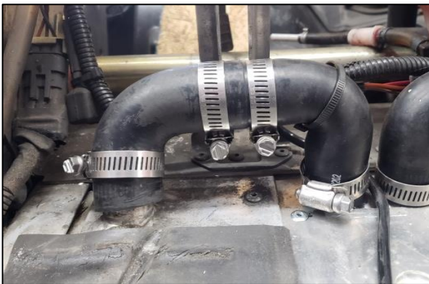
9. Using the provided 2" Aluminum coupler and provided hose clamps, install the provided 90° Hose onto the tunnel cooler then onto the previously cut hose as shown. Tighten clamps.
