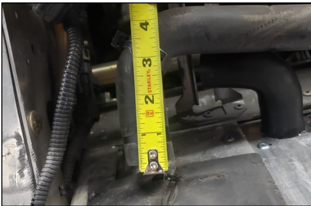
7. Measure, mark, then cut 1" off of the bottom of the PTO Coolant Hose running from the engine to the stock cooler as shown.
