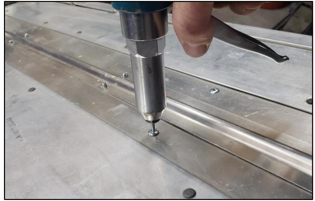
6. Install a rivet in both the front and back sides of the cooler then install the remaining rivets down both sides of the cooler.
