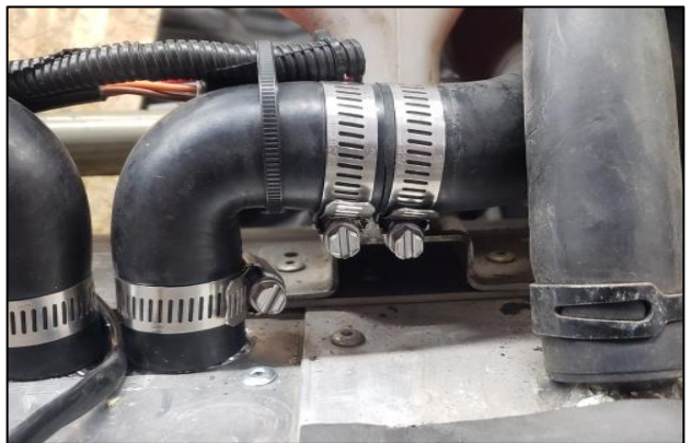
10. Using the other 2" Aluminum coupler and hose clamps, install the provided 90° Hose onto the tunnel cooler then onto the coolant hose coming from the cylinder head. Tighten clamps.
