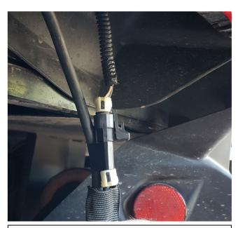
4. Locate the factory tail light connector and plug Blow Hole directly into the tail light as shown.
