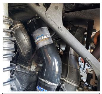
2. Install the Blow Hole by slipping the silicone over the clutch cover intake duct first and then slide the top silicone over the upper duct. Once installed, tighten stock clamps as shown.
