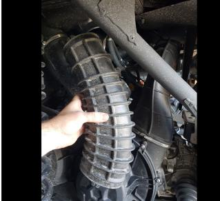
1. Remove clutch intake tube by loosening the clamps on both ends of the clutch intake hose. This clutch intake tube will not be used. Keep the stock hose clamps for later use.
