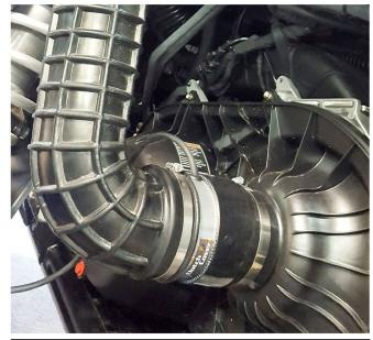
3. Slide Blow Hole over clutch cover. Install clutch intake tube back onto stock intake duct. Tighten clamps. Make sure the intake tube is not touching the shock spring.
