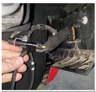
5. Locate the factory tail light connector and plug Blow Hole directly into the tail light as shown. Route wire so it does not rub or chafe.
