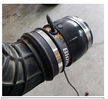
2. Install the Blow Hole inside the clutch intake tube. Heat up the tube and stretch it over the Blow Hole. Make sure the wire is pointed upward as shown.
