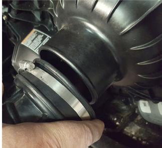
1. Remove the clutch intake tube by loosening the clamps on both ends of the clutch intake hose.
