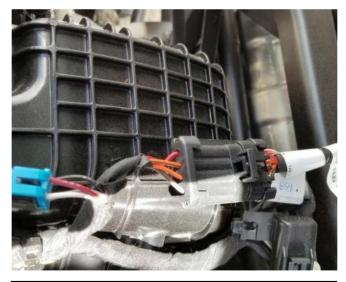
3. Unplug tail light connector and plug in Blow Hole connector in line. Properly route and secure wires and connectors with cable ties as needed to prevent damage.
