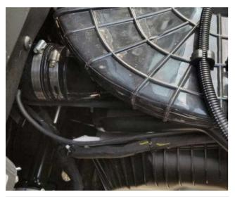
1. Locate the clutch housing intake duct hose. Loosen the clamps holding it onto the clutch cover and remove hose from housing.
