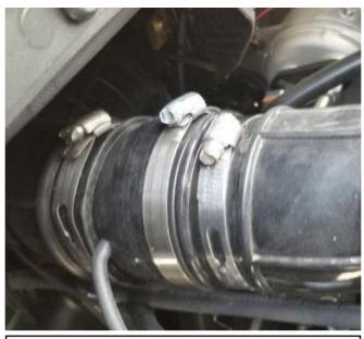
2. Install the Blow Hole onto the clutch housing as shown. Tighten clamp. Then install the intake duct hose onto the Blow Hole assembly. Tighten clamp.
