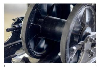
1. Remove the stock rear wheels by loosening the track adjustments bolts and remove the rear axle bolt. Remove the plastic center collar and discard. Remove track adjustment blocks and drill existing axle hole out to %"
