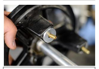
3. Install spacer onto connector bolt as shown.
