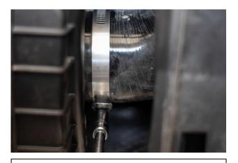
7. Tighten stock clamp on air box and silicone. Make sure everything fits. This may require turning and adjusting the silicone to fit, depending on accessories.
