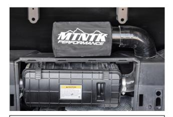
8. Install Pre-Filter as shown with MTNTK Logo facing out. Center the housing between cage tabs above the Pre-Filter. Secure all screws and clamps. Be sure you have removed rag from air box. Reinstall bed access panel.
