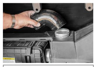
6. Place the aluminum tube inside one of the 90° silicone. Install on air box with aluminum tube showing outside of the hole. Place remaining silicone on aluminum tube as shown.
