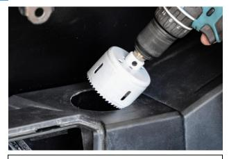
5. Using a 3 ½" Hole Saw, cut the access hole as shown through the plastic console. Deburr the edges and clean all plastic shavings from inside console. Install plastic console back in place.
