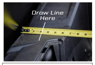
4. Turn tape measure around and measure the width of the plastic console as shown. Measure 3" with a white pen or marker. Use a center punch to mark junction between the two lines.
