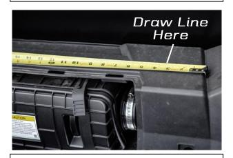
3. Place a tape measure on the top of the plastic console. Measure and mark 3" with a white pen or marker as shown.
