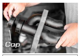
2. Remove the stock air intake plenum and rubber cap from air box as shown. Place a towel or rag inside the air box to keep debris from entering the engine.
