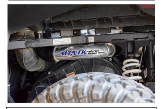
4. Place the new intake tube in the stock location as shown. Secure using the stock clamps. Install the breather hose onto the intake and tighten using stock clamps.
