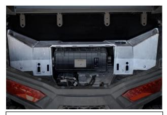
1. Remove access panel from RZR and remove the center console as shown. This requires the removal of the eight torx head screws on the front and back of the cover.
