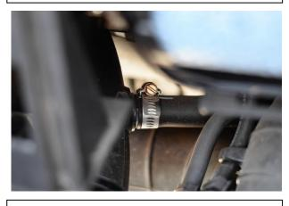
3. Locate the small breather hose secured by a hose clamp and remove. This line will be reattached onto the new intake tube.
