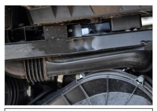
2. Locate the intake tube on the driver's side of the RZR and directly above the clutch cover. Remove the clamps located on both ends of the intake tube. Keep these as they will be used to install the new High Flow Intake Tube.
