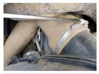
1. Remove Driver's seat. Locate rubber duct located on top of the clutch cover. Loosen hose clamp and remove rubber duct. You will re-use the hose clamp.
