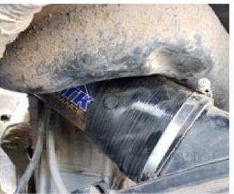
2. Install Blow Hole as shown onto the clutch cover with straight silicone towards the clutch cover. Align MTNTK graphics as shown. This will insure proper routing. Use the stock clamp and fasten the Blow Hole to the clutch cover.
