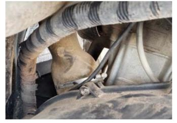
3. Carefully route the Blow Hole wiring harness down the factory harness and under the driver seat towards the front of the machine. Secure wires so they do not rub.
