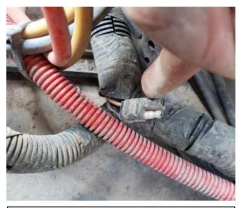
4. Locate the stock accessory plug and insert the Blow Hole harness plug: Red to Orange, Black to White. This allows you to still use the factory accessory plug. Reinstall Driver's seat.
