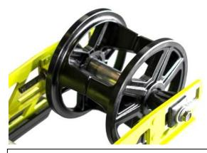
4. Install Tough Wheels onto rear skid in stock location. Align track adjustment collars and bolts. Tighten but do not torque until track is readjusted and aligned. Use the following guide to properly adjust track.
