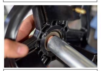
3. Install one spacer each side of the axle collar as shown. Install stock axle between Tough Wheels. Tighten connector bolts.
