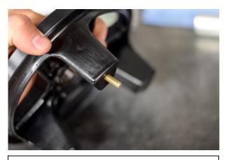
2. Install the stock axle onto the new Tough Wheel. Install the three wheel connector bolts as shown.
