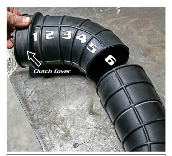
2. Using a silver or white marker, mark section six of the tube as shown in picture. Using a razor blade or knife, carefully cut the entire section (six) out of the intake tube as shown.
