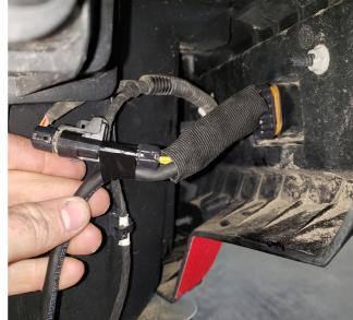
5. Route wiring harness along the bed so it is up and out of the way. Plug directly into the taillight as shown. Be sure the wires will not rub, chafe, or melt. Use zip ties to secure wiring harness.
