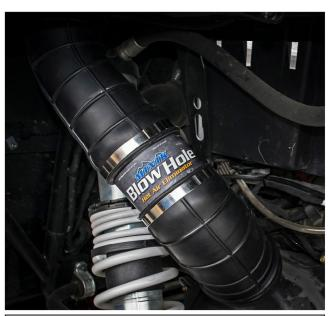
4. Install the intake tube back onto the machine and adjust tubes so wiring harness is towards the machine and logo is facing out. Tighten all clamps.
