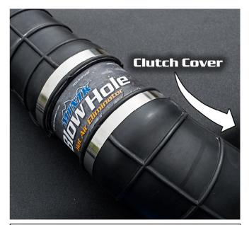
3. Install the Blow Hole and clamps as shown. Slide intake tube onto the Blow Hole as shown. Leave clamps loose for adjustments. This is a tight fit. Use heat and lubrication to install.
