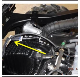
7. Plug in Blow Hole in line. The Blow Hole will run anytime the key is in the "on" position and for a brief 15 second time frame that the ECU keeps the chassis relay powered up after shutdown.
