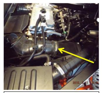
2. Loosen the clamp on the clutch exhaust hose.
