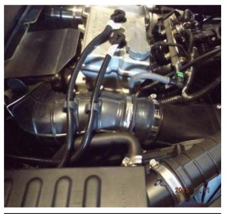
5. Then install exhaust hose onto Blow Hole assembly. Tighten clamp.
