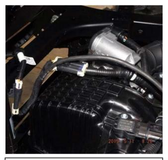
6. Route wire along brake light power cable. Unplug tail light connector.
