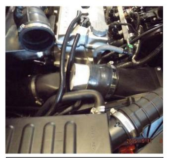
4. Now install Blow Hole onto clutch housing as shown. Tighten clamp.
