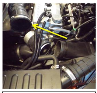
3. Separate the exhaust hose from the clutch housing.
