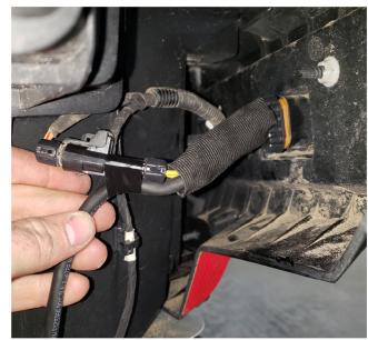
5. Plug harness directly into the taillight as shown. Be sure the wires will not rub, chafe, or melt.
