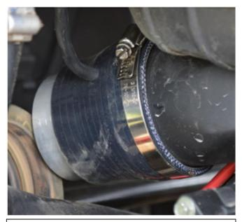
2. Install Blow Hole onto clutch housing as shown by sliding the silicone reducer over the clutch housing. The wire harness should be directed as shown. Tighten clamp.
