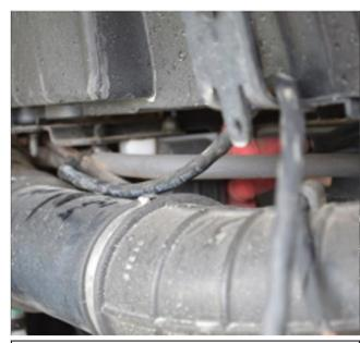
4. Route the wire harness behind the engine intake hose and up to bed support bracket as shown. Use wire ties to secure harness.
