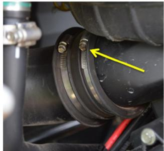
1. Loosen the clamp on the clutch intake duct hose (the end closest to the clutch housing and nearest the front of the clutch housing) and remove from clutch housing.
