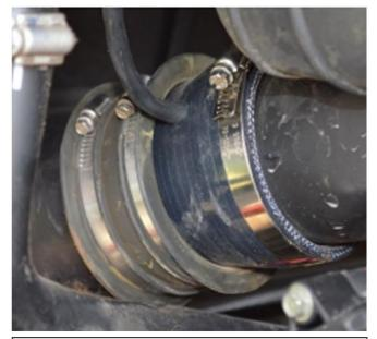
3. Install intake duct hose onto the Blow Hole assembly as shown. Tighten the stock clamp onto the Blow Hole.
