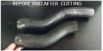
2. Lay the hose down and measure on the opposite end that was marked previously. Mark cut location of the hose @5-1/4". Cut the hose cleanly with a heavy pair of shears or with a razor knife.
