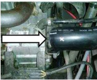
1. Remove seats and rear panel. Locate the clutch intake duct as shown and mark the hose end that goes on the clutch housing (you will need to know this so you can cut the right end off). Remove the hose clamps that hold both ends on and save the clamps.
