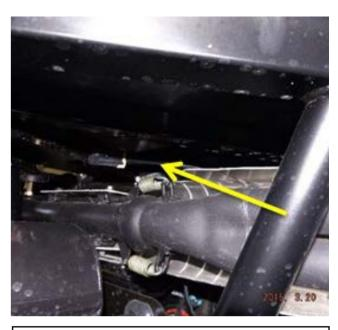
4. Pull excess wire out of the exhaust hose to allow for easy install of Blow Hole.
