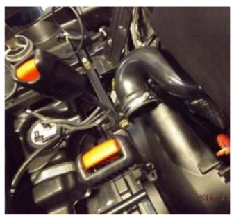
2. Loosen clamp and remove exhaust hose from the clutch housing.
