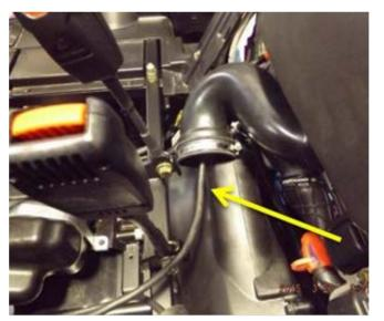
3. Place wiring harness into exhaust hose and route it so it comes out the other end (may need to use some sort of wire to help route it through).
