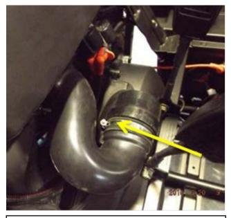
6. Insert metal end of the Blow Hole into the exhaust hose (use of a lubricant may be needed to ensure ease of installation).
