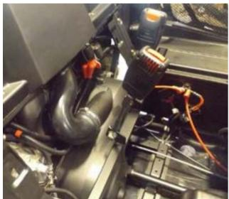
1. Remove the engine access panel located behind the seats, exposing the clutch housing.
