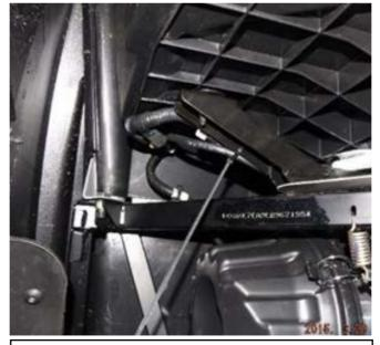
9. Secure wiring to ensure no damage occurs while the RZR is in use. This will also prevent any part of the wiring harness from being exposed to engine components.
