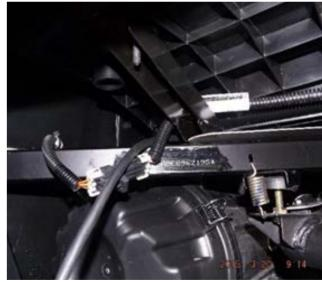
5. Route wiring harness to the driver side of the RZR so you can plug into the tail light harness. Ensure wiring is routed over the support bars to prevent any heating or damage to the wiring.
