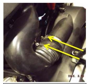
7. Connect silicone end of Blow Hole to the clutch housing and tighten clamp. Ensure the clamps are as shown to prevent the engine access panel from pushing the clamps into the hose.
