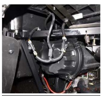
8. Disconnect tail light connection and reconnect wiring harness to proper ends of tail light connectors.
