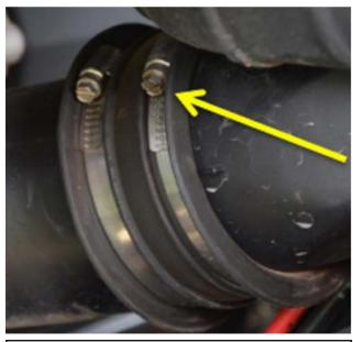
1. To begin, loosen the clamp on the clutch intake duct hose (the end closest to the clutch housing and nearest the front of the clutch housing) and remove from clutch housing.
