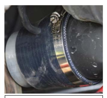
2. Loosen the clamp on the clutch exhaust hose. Separate the exhaust hose from the clutch housing.
