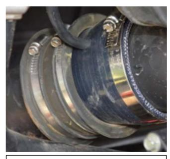
3. Install the Blow Hole onto the clutch housing as shown then tighten clamp. Reinstall exhaust hose onto the blow hole assembly and tighten the clamp.
