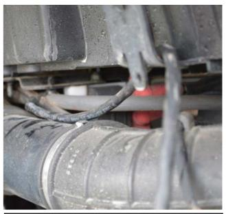
4. Route wire behind the engine intake hose and up to bed support bracket as shown.
