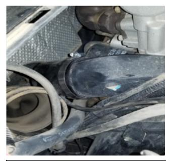
4. Install the Blow Hole onto the plastic clutch intake duct as shown in the picture. The Blow Hole power wire needs to be pointed toward the left – hand side of the machine as shown in picture. Leave the hose clamp loose.
