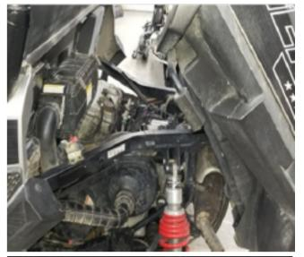
10. Now you can reinstall the outlet duct rubber hose and spark plug wires onto the correct spark plug. Then reinstall the air filter and air filter housing lid. Now is a good time to double check that all wiring and connectors are secured and away from heat and sharp objects.
