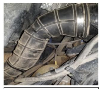
6. Install the two plastic hose clamps onto the hose bends as shown in the picture. These two clamps will keep the hose bends from collapsing and restricting the air flow.
