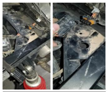
8. Next you need to unplug the bed harness electrical connector as shown in the picture. Remove the female connector from the vehicle frame as shown in picture. Now you will need to remove the plastic retaining clip from the stock wiring connector and install the plastic retaining clip onto the Blow Hole connector.
