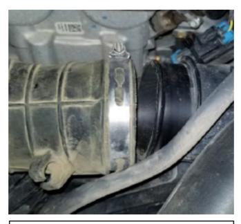
2. Remove clutch box outlet duct hose. Be careful not to lose the metal screen on the end of the hose. Set the hose aside as it will be reinstalled later
