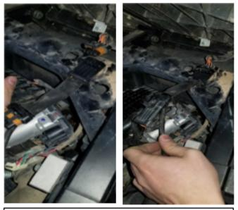
9. The Blow Hole connector will now be held into place on the vehicle frame as show in the pictures. The stock bed harness will now be plugged into the Blow Hole harness. Then you will plug the stock vehicle harness into the Blow Hole harness as seen in the picture.
