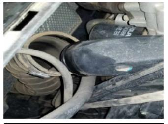
3. Remove the front air intake hose on the clutch box from the plastic duct, as shown in picture.
