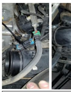
7. Now you will run the Blow Hole wire along side the stock wiring harness towards the rear of the machine. Be sure to route the wire away from any sharp or hot objects. A couple of zip ties will aid in holding the wire in place.
