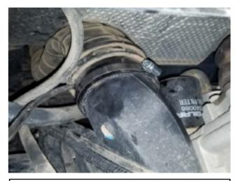
5. Next you will install the stock rubber intake hose onto the Blow Hole. The stock hose will slide over the silicone hose on the Blow Hole,
