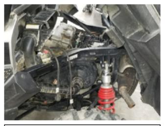
1. To install the Blow Hole, start by raising the bed of your vehicle. Next you will need to remove the air filter lid and spark plug wires from the outlinder band. Days attention to
