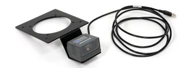
4. Attach the brackets to the head using the screws provided in the standard toolkit.
