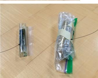
The sealed steel part bag is placed with the other four samples into a larger bag, which is rolled up, sealed, and taped.
