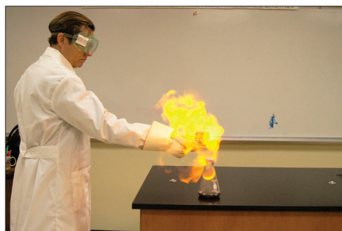
Figure I.8. Energy released as heat and light as hydrogen and oxygen atoms combine to form water molecules.
