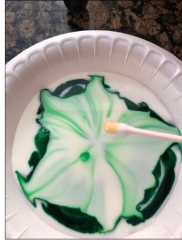
Pattern of dye moving away with the motion of the soap molecules.
