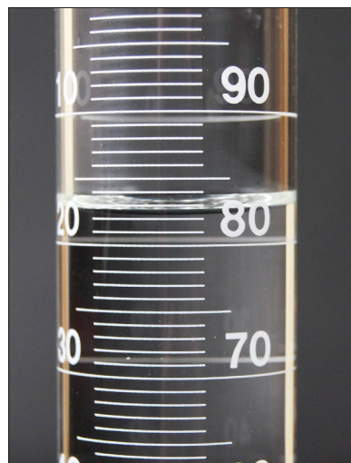
Figure 2.5. Reading the significant digits on a graduated cylinder.
