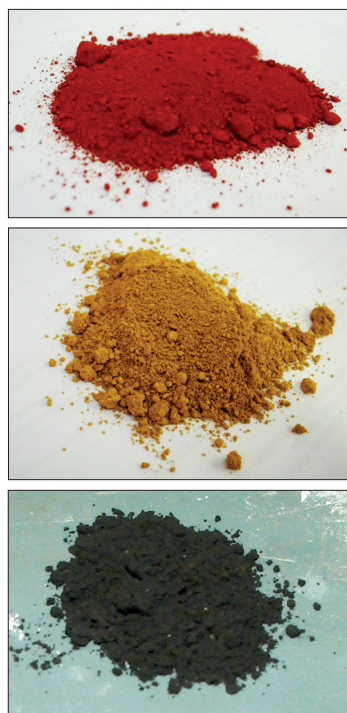
Figure 2.24. Oxides: red iron oxide (top), yellow iron oxide (center), and black copper oxide (bottom).
