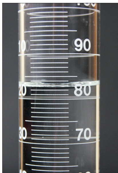
Figure 1.12. Reading the significant digits on a graduated cylinder.
