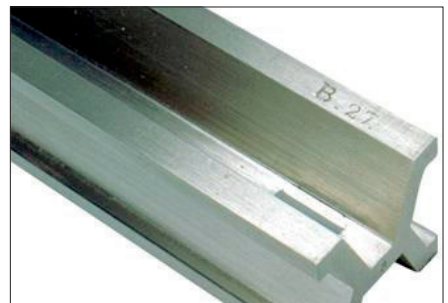
Figure 1.5. Standard meter bar number 27, owned by the U.S. and used as the standard meter from 1893 to 1960.
