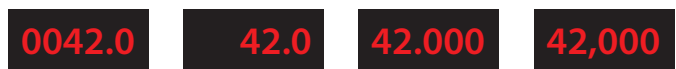
Figure 1.9. With digital instruments, all digits are significant except leading zeros. Thus, the numbers of significant digits in these readings are, from left to right, three, three, five, and five.
