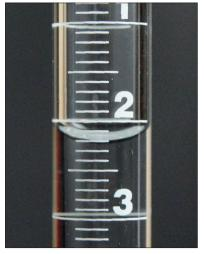
Figure 2.4. Reading the significant digits on a buret.
