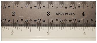
Figure 2.1. The accuracy of these two scales is the same, but the machinist's rule on the top is more precise.
