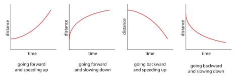
Figure 2.10. Curvature possibilities for distance vs. time graphs.
