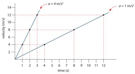
Figure 2.7. A plot of velocity versus time for an object accelerating uniformly. Two different acceleration cases are shown.
