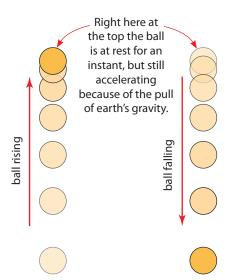
Figure 2.8. A rising and falling ball illustrates the difference between velocity and acceleration.
