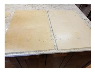
9) Rotate the partially assembled cabinet body so that the finished edges face down onto your work surface and attach one side panel to the cabinet body with 5 steel locking caps, ensuring that the finished edge faces the same way as the body. The sides should only fit one way, and it does not matter if you start with the left or right side of the cabinet.
