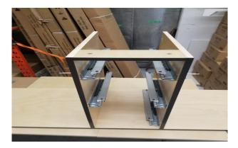
4) Rest the lower drawer slides on the floor panel under the ones previously affixed, ensuring that all slide rails face the same way, and use a ruler or level to make sure that they are the same distance from the front face of the gable, then affix the bottom slide rails to the drawer gables using #6 x 5/8 wood screws, then place 4 wooden dowels in the appropriate holes on the top rear of the drawer gables
