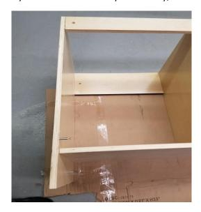
10) Locate and dowel the finished toe kick panel and lower rear support brace. Affix these to the side panel you just attached to the cabinet body using 2 steel locking caps. Ensure that the finished face of the toe kick faces the same was as the finished edges of your cabinet body so it will be visible when the cabinet is upright.
