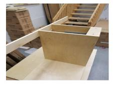
6) Locate and dowel the 2 finished face plate mounting boards. Affix them to the front locking pins on the top of the gables, ensuring at the finished face is forward and the long finished edge faces down into the cabinet body.
