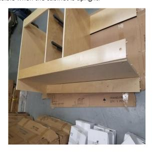
11) REPEAT STEP 9 TO ATTACH THE REMAINING SIDE PANEL TO THE CABINET BODY AND DOUBLE CHECK TO MAKE SURE THAT NO LOCKING CAPS HAVE BEEN MISSED AND THEY HAVE ALL BEEN TIGHTENED APPROPRIATELY
