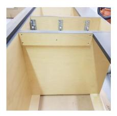
8) Locate the 2 side panels of the vanity, they should be the largest remaining pieces with finished outsides, place them finish down and spine to spine on your work surface and affix steel locking pins into all available white receptacles in both side panels.
