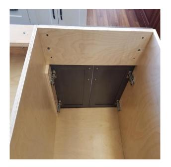
Remove the spring clamps and paint stick and your new 60" double sink vanity is now complete and ready for installation. It is a good idea at this point to thoroughly vacuum out the entire cabinet to ensure that no sawdust or splinters from drilling can get into the drawer slides as over time they may potentially inhibit the proper operation of the slides and / or door hinges.
