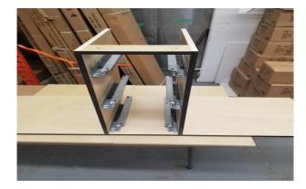
5) Locate and dowel the upper horizontal support brace, affix steel locking screws into the receptacles along the one side of the brace, and insert 4 wooden dowels into the appropriate holes in the end of the brace. Insert the locking screws into the holes on the top rear of the gable above the drawer slides and secure with steel locking caps
