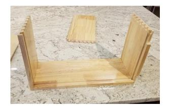
17) Insert the floor panel into the groove, ensuring the varnished surface faces the top, and drop the grooves on the last side panel into place to complete the drawer box. If need be, gently tap the tabs into the grooves of the dove-tail joint with a rubber mallet until the edges are flush
