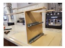
5) Locate the cabinet door bump-out panel and affix to the inside of the centre gable (opposite the drawer slides) using 5 - #6 x 1 ½" wood screws, ensuring that the finished edge faces outward and is flush with the finished edge of the centre gable
