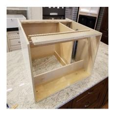
11) **IF YOU ARE ATTACHING THE OPTIONAL DECORATIVE TOE KICK PANEL**, stand the cabinet body up upside down, locate it and clamp it to the outer finished surface of the flat toe-kick so that the corners are flush with those of the cabinet. Mark a pencil line along the inside edge of the toe kick panel
