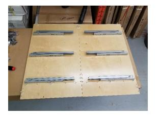
9) Rotate the partially assembled cabinet body so that the finished edges face down onto your work surface, carefully align the locking caps. It does not matter which side you start with, however, be sure that the finished edge of the side panel faces down like the cabinet body and that the drawer slides face down as well. Side panels should only fit onto the cabinet body one way.
