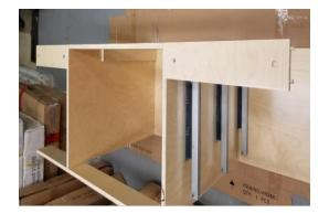
6) Locate and dowel the upper rear support brace. Affix 2 steel locking pins to the white receptacles along the brace and affix it to the upper rear of the drawer gables using 2 steel locking caps.
