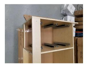
10) Locate and dowel the lower rear support brace and the finished toe kick panel. Affix these pieces to the previously attached side panel using 1 steel locking cap per piece. Ensure that the finished face of the toe kick panel faces down toward your work surface so that the finish will be visible when the cabinet is upright.
