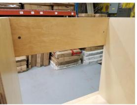
4) Rest the bottom drawer slides on the floor panel under the 4 previously affixed, ensuring that the slide rails face the same way, and use a ruler or level to make sure that they are the same distance from the front face of the gable, then affix the last 2 slide rails to the drawer gables using #6 x 5/8" wood screws, then place 4 wooden dowels in the appropriate holes along the top rear edge of the gables.
