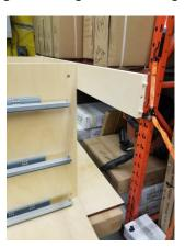
7) Locate the cabinet door bump-out panels and affix to the inside of the centre gables (opposite the drawer slides) using 5 + #6 x 1 ½" wood screws per panel (10 total), ensuring that the finished edges face outward and are flush with the finished edges of the drawer gables.
