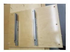
REPEAT UNTIL YOU HAVE ATTACHED 4 SLIDES (2 PER GABLE) TO THE UPPER AND MIDDLE ROWS OF PILOT HOLES IN BOTH DRAWER GABLES, DO NOT ATTACH THE BOTTOM SLIDES YET.
