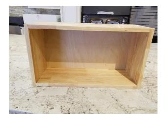
18) With the drawer box face down, ensure that the box is square using a roofing square, and affix the adjustable slide-retention clip in the front-most corner of the bottom of the drawer using 2 - #6 x 5/8" screws per clip (4 in total)
