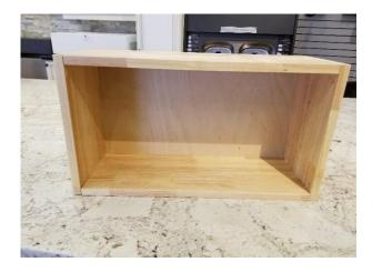
18) With the drawer box face down, ensure that the box is square using a roofing square, and affix the adjustable slide-retention clip in the front-most corner of the bottom of the drawer using 2 - #6 x 5/8" screws per clip (4 in total)
