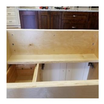
Remove the spring clamps and paint stick and your new vanity is now complete and ready for installation. It is a good idea at this point to thoroughly vacuum out the entire cabinet to ensure that no sawdust or splinters from drilling can get into the drawer slides as over time they may potentially inhibit the proper operation of the slides and / or door hinges.
