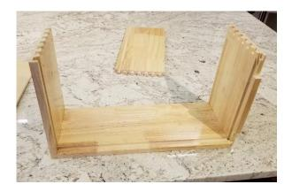
17) Insert the floor panel into the groove, ensuring the varnished surface faces the top, and drop the grooves on the last side panel into place to complete the drawer box. If need be, gently tap the tabs into the grooves of the dove-tail joint with a rubber mallet until the edges are flush
