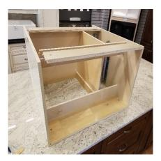
11) Stand the cabinet body up, upside-down, and if you are attaching the decorative toe-kick panel, locate it and clamp it to the outer finished surface of the flat toe-kick so that the corners are flush with those of the cabinet. Mark a pencil line along the inside edge of the toe kick panel
