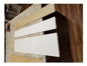
8) Align the appropriate steel locking pins in the right side panel with the holes in the bottom and 2 upper support braces of the cabinet body, ensuring that all 4 drawer slides are facing the same way and that the edge tape on the side panel faces down. Insert the pins into the holes and secure the panel with 5 steel locking caps
