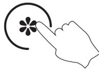
Press the airflow button and the airflow display area displays "3" and works in high gear; press again, the airflow display area displays "2" and works in medium gear; then press once, the airflow display area displays "1" and works in low gear; press the button again, the airflow display area displays "0", and the fan will stop working. The buzzer sounds every time you press the button.
