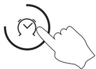
Press the "Timer" reminder button once, the timer display area displays "1", indicating that the timing is 10 minutes. The range hood will give the tone to remind the user the time set is up. If the button is pressed twice, the timer display area displays "2", indicating that the timing is 20 minutes by that analogy. A maximum of 60 minutes is allowed. After the time set is up, press any key to cancel the timer tone.
