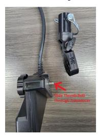
Then screw into transducer Mount and hand tighten.
