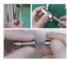
6. Twist out the rear cover of the movement with 4# tooling and take out the movement.
