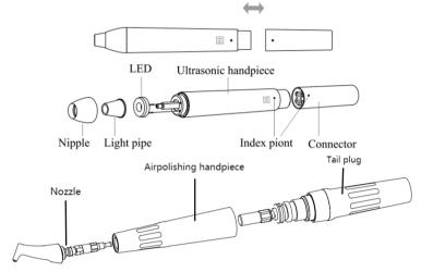
Figure 9 Ultrasonic handpiece and Air polishing handpiece
