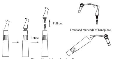
Figure 8 handpiece cleaning diagram
