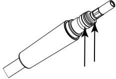
2. Sand pipe at the bottom of the main engine: there is an on-off valve to control the sand powder on and off at the bottom of the main engine, and the sand pipe at the on-off valve may be damaged for a long time; it needs to be replaced after damage. Expected life of sand pipe at the bottom:
