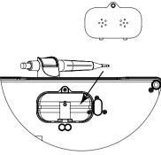
3. The sandblasting tail line of the main engine: there is a sand hose in the tail line of the sandblasting handpiece, and the wear of the hose for a long time may lead to air leakage and sand leakage of the tail line; it needs to be replaced after damage. Expected life of sand pipe at the bottom:
