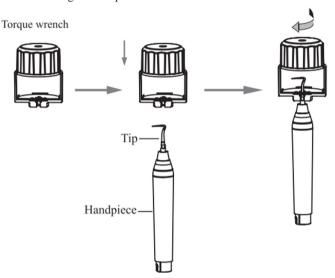
Figure 5 Installation diagram of tip
