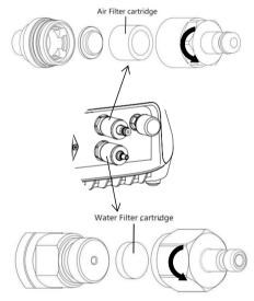
Fig. 10 schematic diagram of filter replacement
