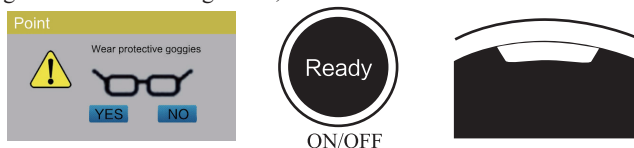
Figure 20 Schematic diagram of prompt of wearing glasses, Ready state, and green indicator
