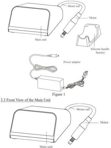
It mainly consists of main unit, motor, power adapter, etc.
