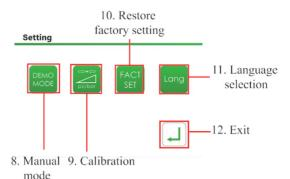
5.7.1 In setting interface, touch key "8" Manual Mode key to enter manual mode interface. Under the manual mode state, the rotation of motor can be directly controlled without foot pedal. Touch Speed Ratio key to select corresponding speed ratio. Touch Speed key to adjust the speed. Touch Start key, Stop key, Forward/Reverse Rotation key, and LED key to control the output of motor. Touch the Exit key to exit the manual mode interface.
