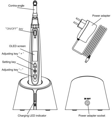
The version of software is displayed on the OLED screen when starting up.
