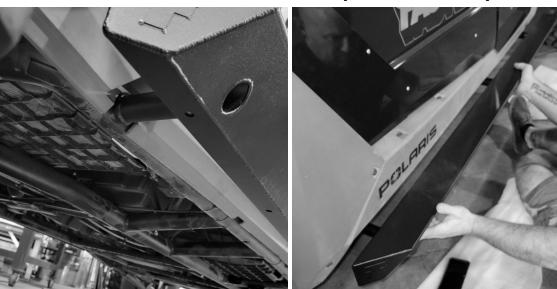
3) While one person holds the Slider in place, the other can slide the bolts into place. Use a shallow 19mm or ¾ socket with an extension to push it through the tube. Apply some thread locker to each bolt before threading on the nut insert.
