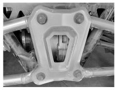
3) Install the new Fastlab Pull Plate by sliding a bolt through the pull plate and radius rod then into the frame. Move the tires around if you need to align it to the frame. Put a nut onto each bolt once you get it through to make sure it does not back out. For Turbo R models, transfer the upper bushing heat shield to the Fastlab Pull Plate. Torque all bolts to factory spec.
