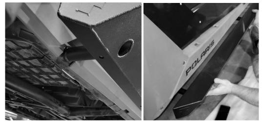
3) While one person holds the Slider in place, the other can slide the bolts into place. Use a shallow 19mm or ¾ socket with an extension to push it through the tube. Apply some thread locker to each bolt before threading on the nut insert.
