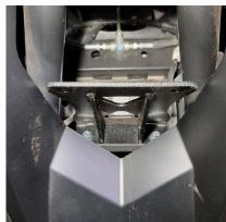
2) If the hood was removed, tighten the 6mm bolts and reinstall it. Now, attach the upper bracket to the lower bracket with the supplied 5/16" nuts and bolts. Once that is complete you can mount your choice of pods or light bars to the upper bracket slots.
