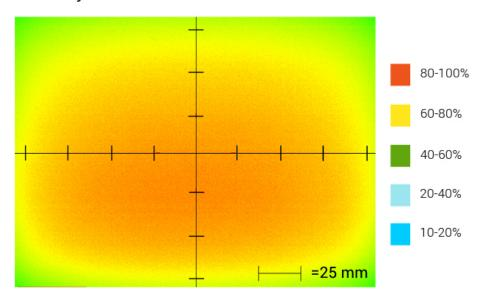
Optical measurement taken using DL067A12-WHIIC Rev. A @ 25mm
