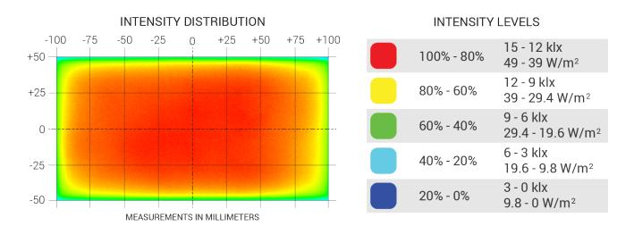
OPTICAL MEASUREMENTS TAKEN AT THE DIFFUSER SURFACE USING 4" x 8" WHITE LED MODEL
