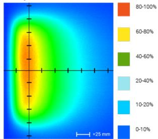
Optical measurement taken using AL4554-660C5 @ 25mm
