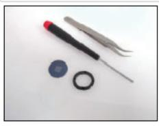
Screwdriver or tweezers are recommended to remove retaining ring, but are not included. Retaining Ring will turn clockwise to install and counter-clockwise to remove. There are two small holes and two slots in ring to install/remove. Install the shiny metal side of pattern towards the LED
