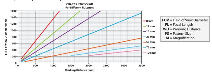
To estimate the Focal Length (FL) required for Working Distance (WD) and Field of View (FOV).
