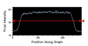
The ODRD130 offers a very diffuse light pattern at a defined working distance between 150mm – 450mm. The Pixel Graph representation shows a steep drop off in intensity outside of the active area with a very diffuse light pattern inside.
