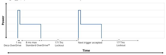
The duty cycle of Dual OverDrive on the JWL225-DO Series is 5%.
