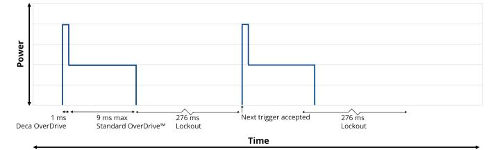
The duty cycle of Dual OverDrive on the JWL150-DO Series is 3.5%.
