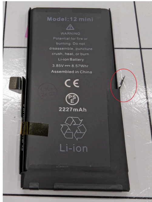
iPhone 12 Mini Battery with additional connector highlighted
